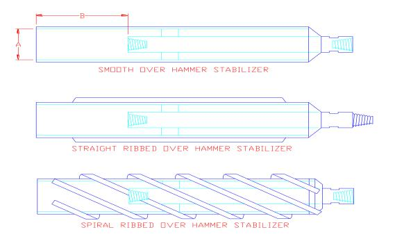
In building a stabilizer we will build the stabilizer ID, dimension A above, to fit the case diameter. The case housing length, dimension B above, is the length of the stabilizer case over the hammer. These dimensions must be specified.
